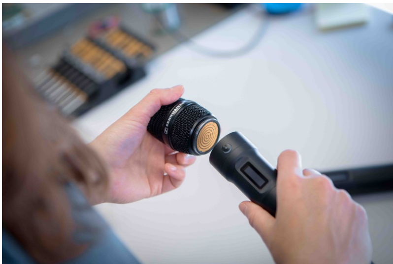
The Command adapter for the Spectera SKM adds a talkback channel for the field reporter, for example
